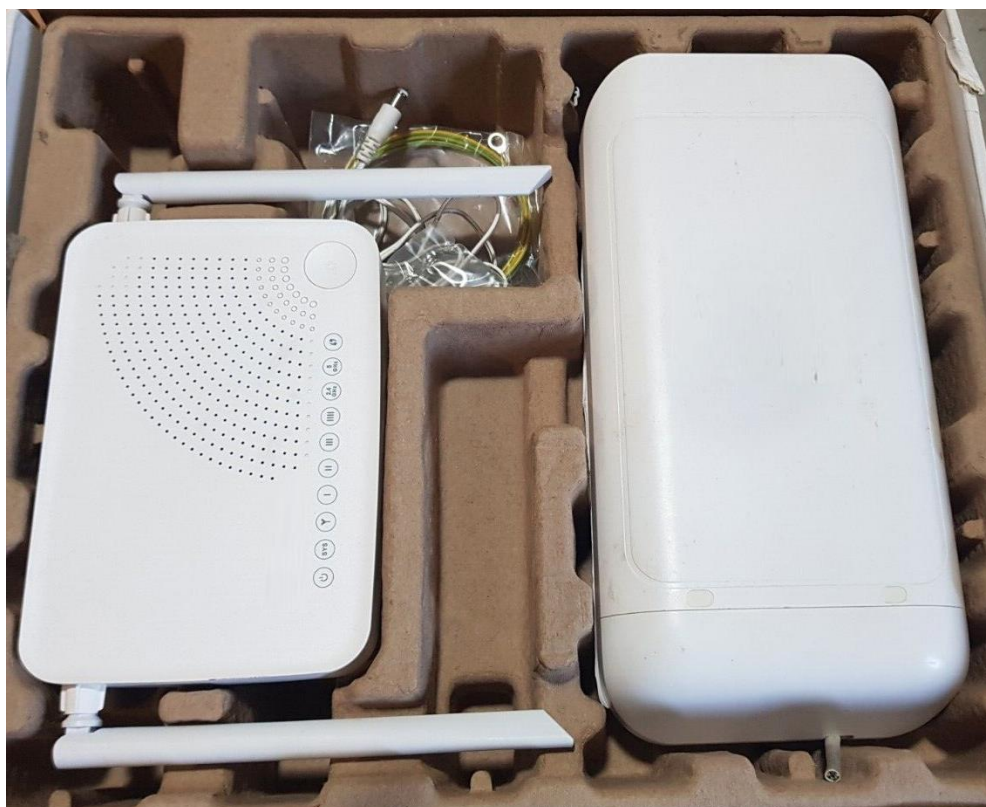
Figura 1: Kit Fornito. Router/Antenna e Apparato Access Point Micro Business
